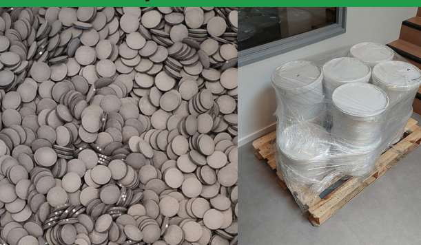
TCM tablets ready to fill the battery for further test
