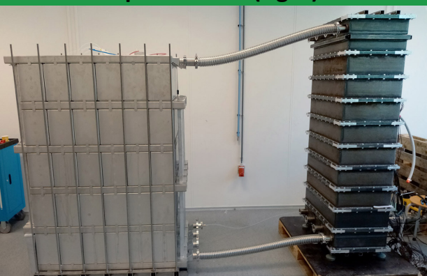
First tests of the connected TCM module (left) and the component box (right)
